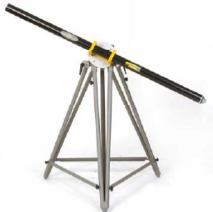
figure 7: The K-Reference Bar + tripod
