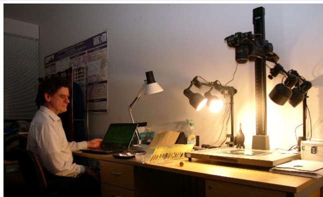
Fig. 3. Copystand with four tungsten-halogen lamps for reflective imaging of samples with the Nikon D200 camera. The filter is screw-mounted into the front of the lens.
