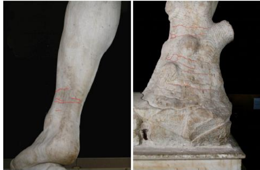
Figure 1: The two images show the regions affected by the fractures (the back of the left leg and the so-called "broncone", i.e. the tree stump on the back of the right leg), most of them extremely thin. Images courtesy of A. Borri (BORRI et al, 2004).
