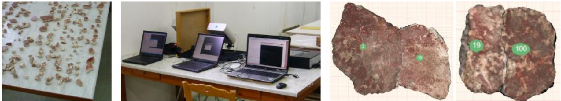
Figure 1: Our acquisition system, deployed at the Akrotiri Excavation, Thera. We use a flatbed scanner to capture high-resolution images and normals of wall painting fragments (shown at left), and multiple 3-D scanners to acquire geometry. A single user can operate up to four scanners simultaneously, while a second user operates the flatbed scanner and verifies processing results. This yields a throughput of approximately 10 fragments per hour. Our matching algorithm correctly finds the only two matches in this data set using the scanned 3-D geometry.
